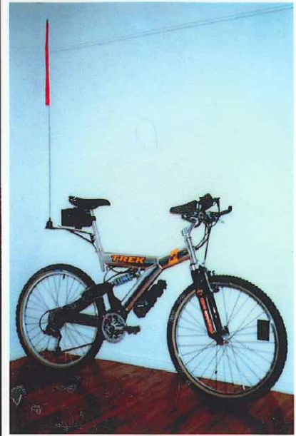
KE4WMF's bicycle-mobile station—a TREK mountain bike customized for 2-meter FM operation. That's a gel-cell battery under the seat and the radio is mounted to the handlebars.
