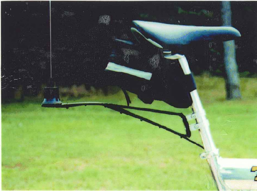
Close-up view of the antenna mount. The antenna is an unmodified Larsen NMO-150HW 1/2 -wave vertical, which does not need a ground plane. The mount is "homebrewed" from solid aluminum rod and held together with Goop household glue.
