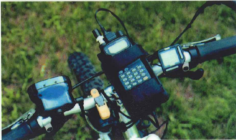
Detail of the author's hi-tech handlebars. To the left of the HT is his 115-dB air horn, and over on the right is his "Radar cyclocomputer," which reads out more information than most automobile dashboards.
