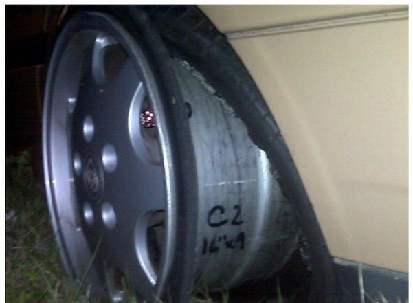
ABOVE. Some lightweight wheels even develop tiny cracks which slowly let air out of the tire, giving the appearance of a hazard-induced blowout when the tire actually failed due to under-inflation. New England has some of the worst roads I've ever driven on. I once struck a pothole with so much force that it sent a rear strut into the passenger compartment! However, there was no blowout or bent wheel. Make smart wheel/tire purchases or learn to live with the consequences!
